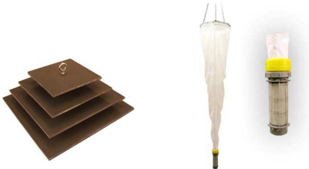
Figure 6: Zebra mussel sampling equipment purchased by the program for monitoring kits including Multi-plated Masonite samplers (left) and veliger nets (right)
